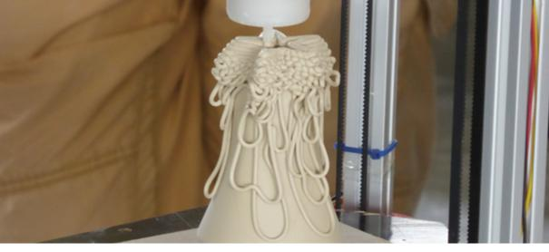
32 Özgündogdu (2015), p. 14 33 Johnson (2011) top: Fig. 4 3D printing directly onto a freshly slip cast lid for a sugar bowl. Photo: Tapio Yli-Viikari right: Fig. 5 A replaced 3D printed handle right: Fig. 5 A replaced 3D printed handle factory.
